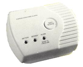
by heat producing devices (e.g., furnaces, hot water tanks), and rises with the heat. CO detectors must be located not less than 15 feet, nor more than 30 feet, from gas-fired heat-producing devices. Ideal spacing is 15 – 20 feet, and never *above* a heat producing device.
