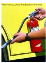
**A = AIM** Aim the extinguisher and the hose for the *base* of the fire. **Remember:** the base of the fire is the leading edge and the lowest *visible* point of the flame. Did you get it right?
